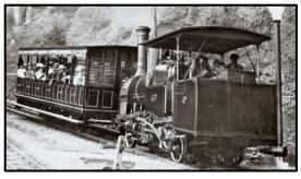
**Figure 6: Rigi rack-and-pinion railway** Source: http://www.rigi.ch/Company/Rigi-Bahnen/ Railway-and-mountain-history
